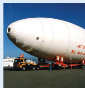
Airship constructed with VECTRAN
