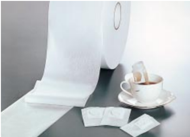
Coffee bags made from a melt-blown nonwoven fabric
